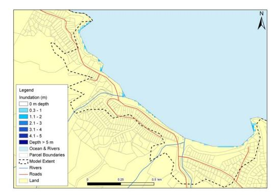
Figure 55: Langs Beach, Bream Bay: Maximum inundation speed (upper) and depth (lower) plots for the Mw8.5 Tonga-Kermadec subduction zone scenario at MHWS + 50cm (to extent of LiDAR).
