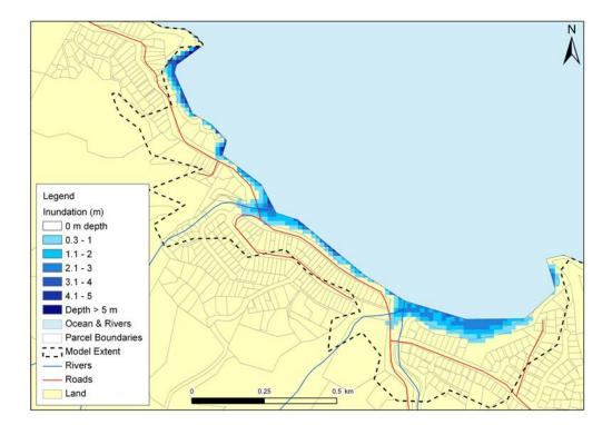
Figure 56: Langs Beach, Bream Bay: Maximum inundation speed (upper) and depth (lower) plots for the Mw9.0 Tonga-Kermadec subduction zone scenario at MHWS (to extent of LiDAR).
