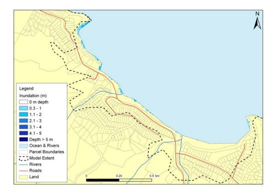
Figure 54: Langs Beach, Bream Bay: Maximum inundation speed (upper) and depth (lower) plots for the Mw8.5 Tonga-Kermadec subduction zone scenario at MHWS (to extent of LiDAR).
