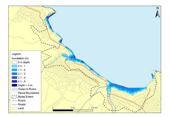
Figure 53: Langs Beach, Bream Bay: Maximum inundation speed (upper) and depth (lower) plots for the South American tsunami scenario at MHWS + 50cm (to extent of LiDAR).
