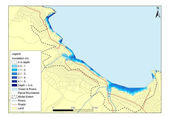
Figure 57:Langs Beach, Bream Bay: Maximum inundation speed (upper) and depth (lower)plots for the Mw9.0 Tonga-Kermadec subduction zone scenario at MHWS + 50cm<br/>(to extent of LiDAR).
