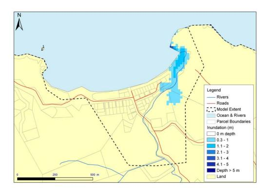
Figure 61: Te Ngaire, Whangaroa: Maximum inundation speed (upper) and depth (lower) plots for the Mw8.5 Tonga-Kermadec subduction zone scenario at MHWS + 50cm (to extent of LiDAR).
