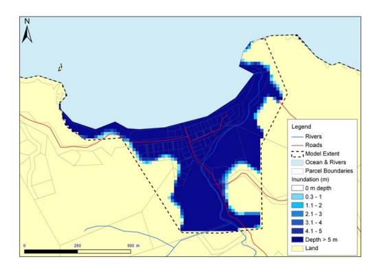
Figure 62: Te Ngaire, Whangaroa: Maximum inundation speed (upper) and depth (lower) plots for the Mw9.0 Tonga-Kermadec subduction zone scenario at MHWS (to extent of LiDAR).
