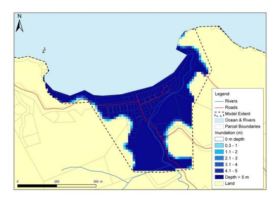
Figure 63: Te Ngaire, Whangaroa: Maximum inundation speed (upper) and depth (lower) plots for the Mw9.0 Tonga-Kermadec subduction zone scenario at MHWS + 50cm (to extent of LiDAR).
