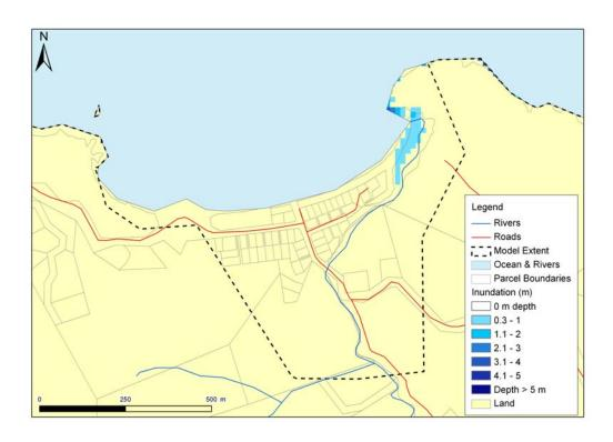
Figure 60: Te Ngaire, Whangaroa: Maximum inundation speed (upper) and depth (lower) plots for the Mw8.5 Tonga-Kermadec subduction zone scenario at MHWS (to extent of LiDAR).
