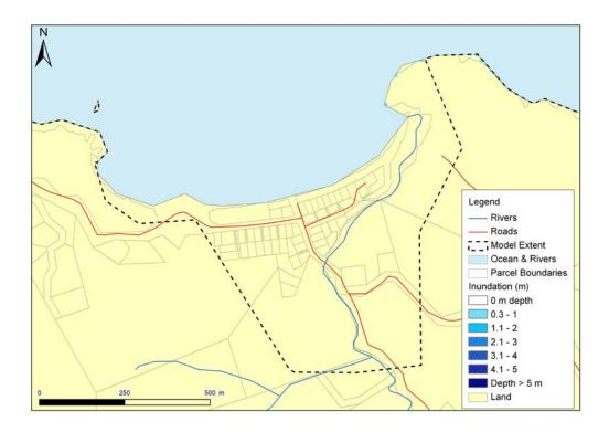
Figure 58: Te Ngaire, Whangaroa: Maximum inundation speed (upper) and depth (lower) plots for the South American tsunami scenario at MHWS (to extent of LiDAR).
