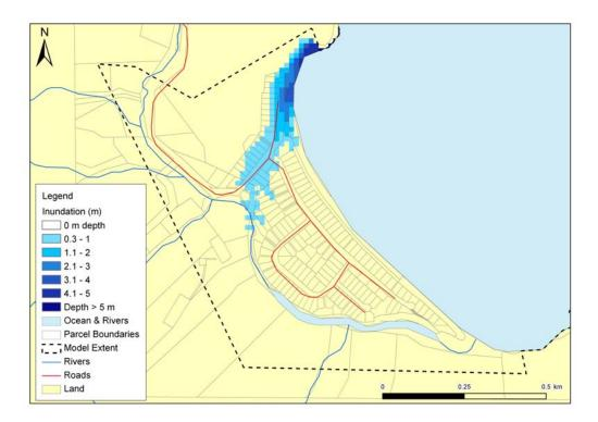
Figure 42: Taupo Bay, Whangaroa: Maximum inundation speed (upper) and depth (lower) plots for the  $M_w8.5$  Tonga-Kermadec subduction zone scenario at MHWS (to extent of LiDAR).
