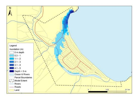
Figure 43: Taupo Bay, Whangaroa: Maximum inundation speed (upper) and depth (lower) plots for the  $M_w8.5$  Tonga-Kermadec subduction zone scenario at MHWS + 50cm (to extent of LiDAR).
