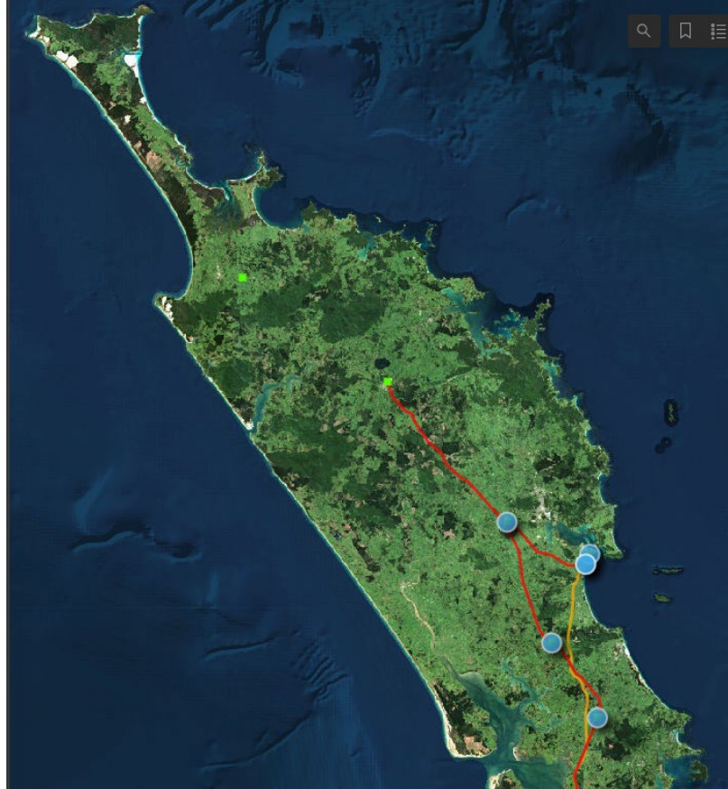
Figure 1. Map of Northland showing national grid assets (blue dots and green squares represent substation locations, red lines represent 110kV lines, and orange lines represent 220kV lines)
