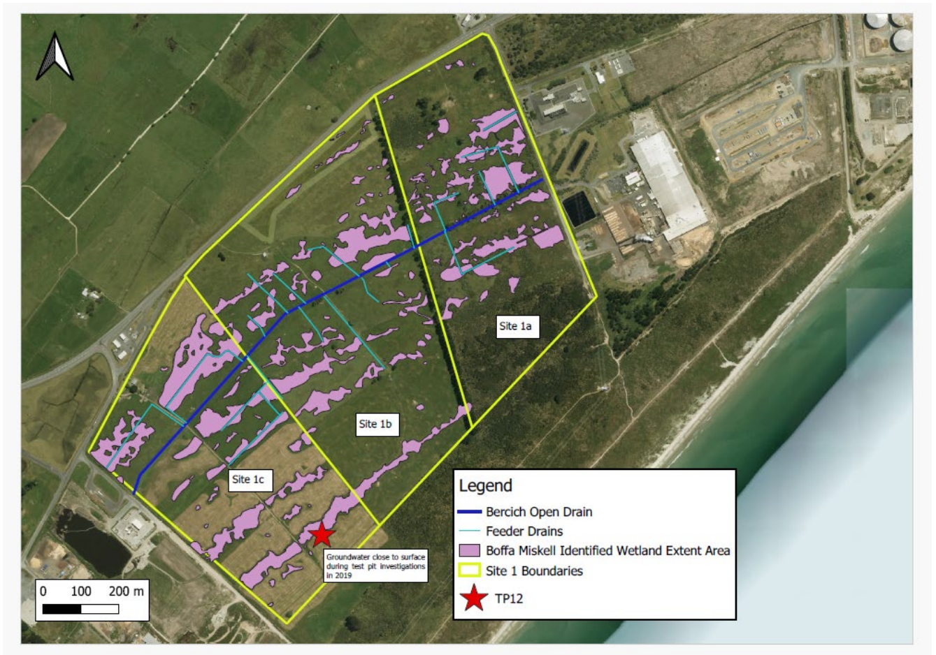
Figure 1 shows the Bercich Drain (in dark blue), feeder drains in light blue and location of TP12 where groundwater was identified close to the surface in test pit investigations in November 2019 (Source: Boffa Miskell, Nov 2023).
