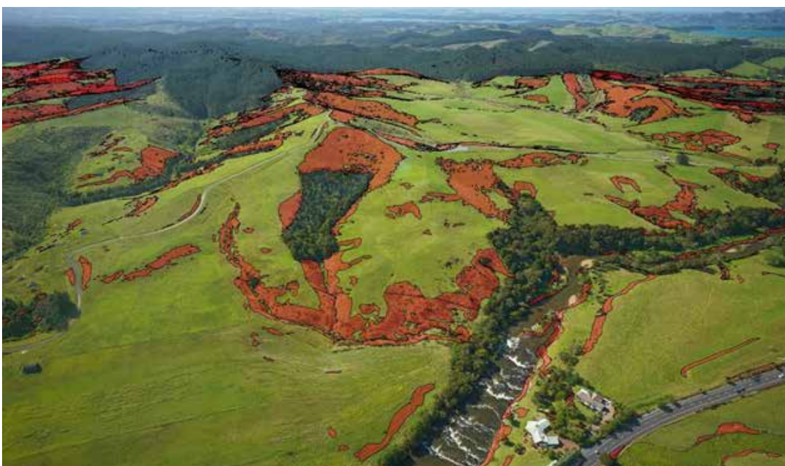
Indicative erosion risk is shown in a red layer overlaid on oblique aerial imagery. Source: NRC
