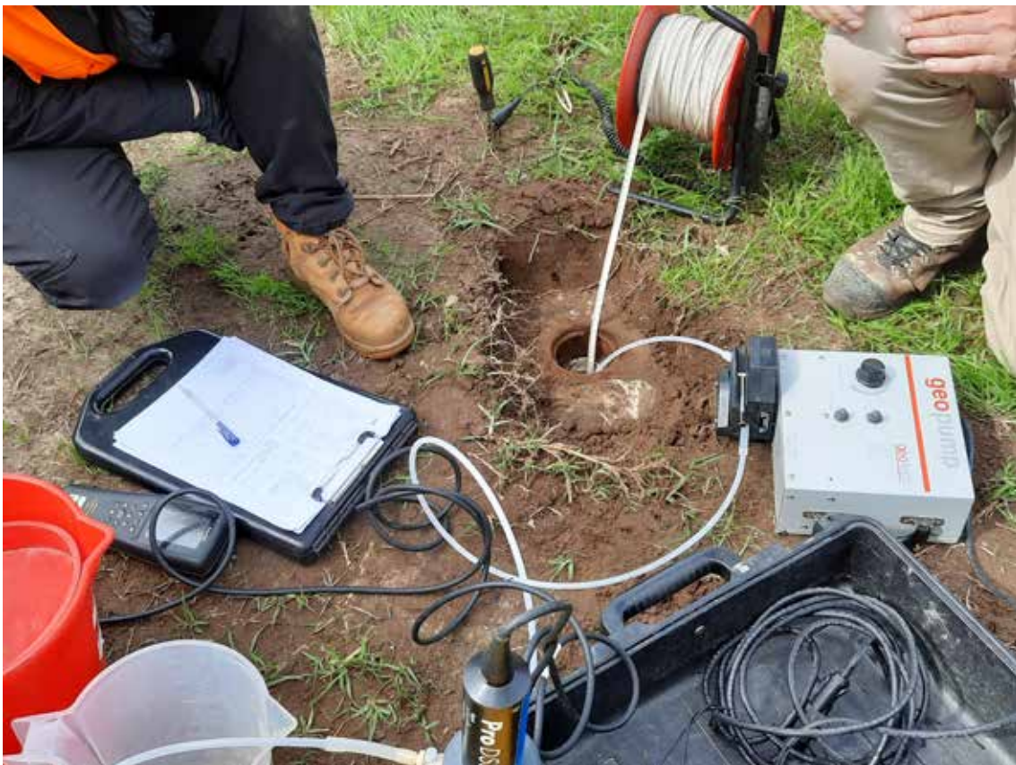
NRC staff sampling from a bore to monitor levels of contaminants in the environment.
