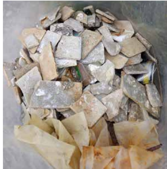
Example materials that contain asbestos.
