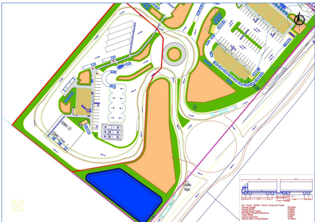
Figure 15: Typical tracking paths for a 23m HPMV truck and trailer
