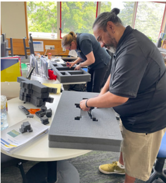
Members of Northland CDEM hand-cut the foam to make custom, weather-proof cases for Starlink units
